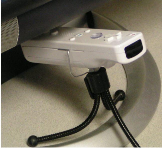
Figure A.1: Nintendo Wii remote positioned under computer monitor.
