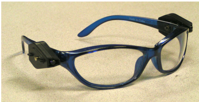
Figure A.2: Safety glasses with infrared LEDs mounted to the sides.
